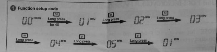
Once you find your desired spark plug firing pattern, release the S1 button. The default for the standard model is 02(once per revolution).
